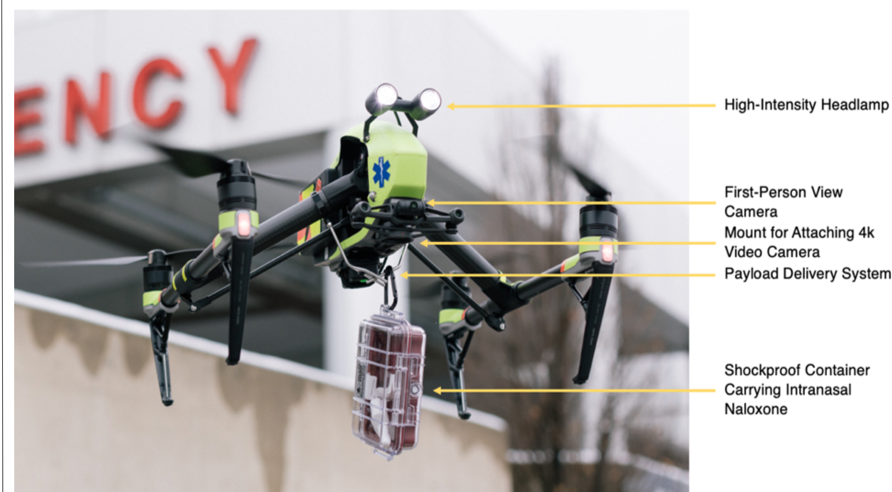
Figure 1: Customized DJI Inspire 2 drone used for this study.
